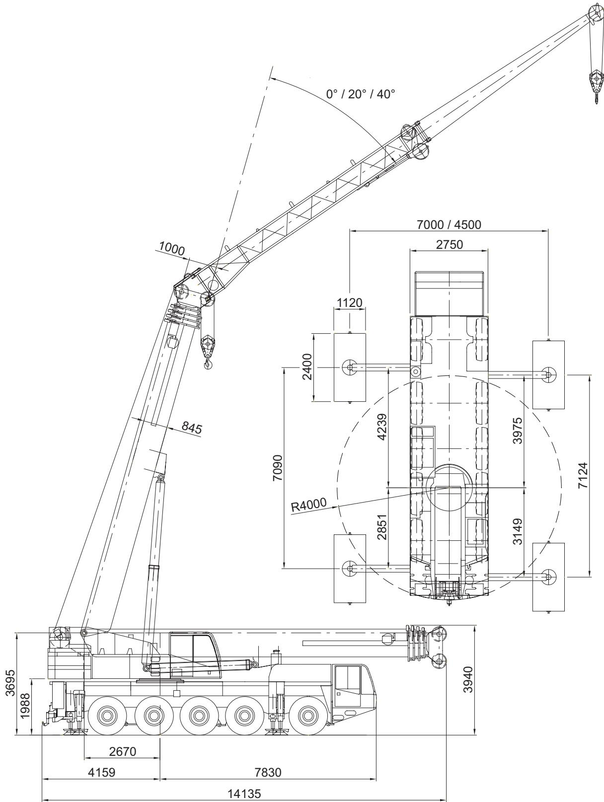
Dimensions are in millimeters.
